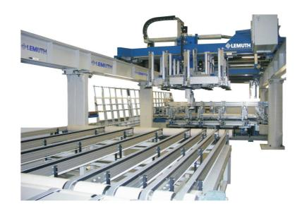
In this configuration, the glue is usually applied to the inside or the outside of the sash overlap. High-precision handling units fully automatically perform all work processes such as loading the sash, applying the glue and inserting the glass in a precise manner. Because it is mainly wooden sashes that are glued in the overlap, the sash can be aligned precisely at right angles by means of the clamping table. Once the glue has set, the aligned sash will retain its shape permanently.
