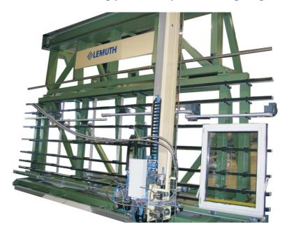
When the glue is applied in the sash rebate, it is applied between the glass pane edge bond and the sash profile. A gap of approximately 3 mm is required for this application. For the gluing of the glass pane, the sash can already be mounted in the frame. The advantage of this is that the sash can be optimally aligned in the frame. Thanks to the increased rigidity of the sash after gluing, the sash and the frame form a perfect unit.
